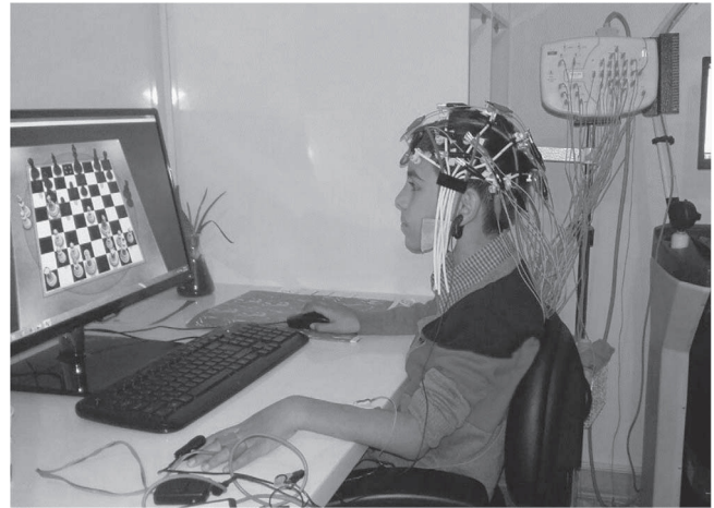
Fig. 1. Data acquisition setup. Subject engaged in chess against a computer. The subject reported six episodes of critical decision making during which a real-time EEG recording was marked and subsequently grand averaged in brain mapping. The galvanic skin conductance (GSC) and heart rate variability (HRV) were simultaneously monitored during the procedure with special markings indicating decision making episodes.
