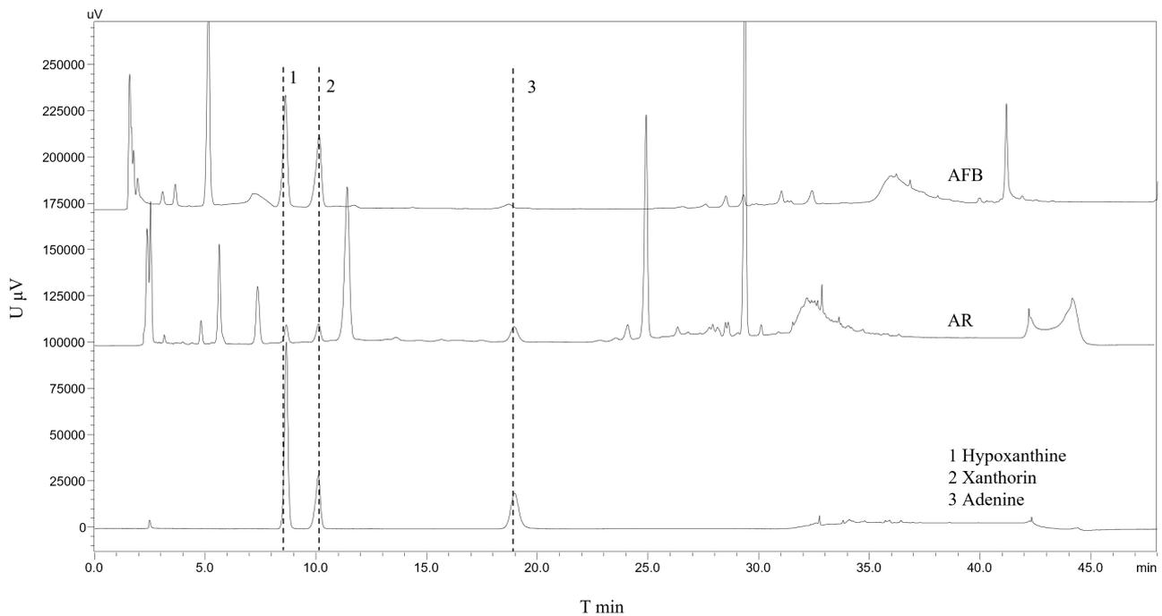
**Fig. 1. Liquid Chromatogram of Samples and Standards.** 1: hypoxanthine; 2: xanthine; 3: adenine.
