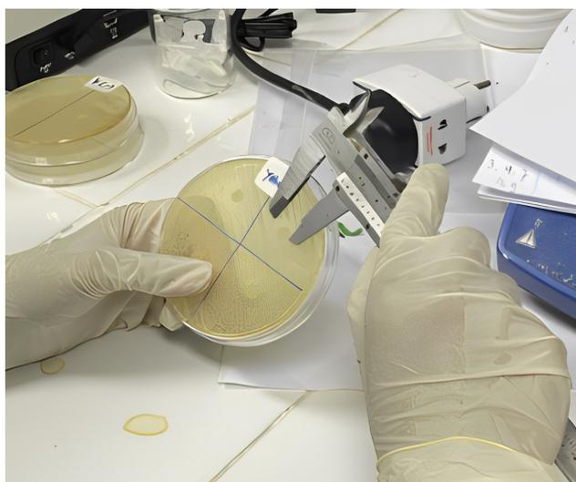
**Fig. 4.** The diameter measurement of the inhibition zone in each testing group was conducted with a Vernier caliper in millimeters.
