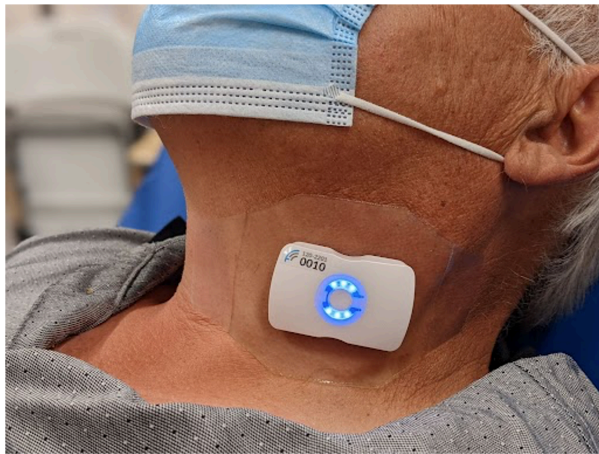
Fig. 1. The wireless, wearable Doppler ultrasound system. (A) The device on the neck of a volunteer. (B) The graphical user interface of the ultrasound system displayed on an iOS device.
